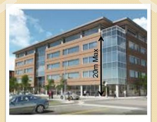
No portion of the required Fire Access route to be more than 20m below the floor level of the uppermost storey.
